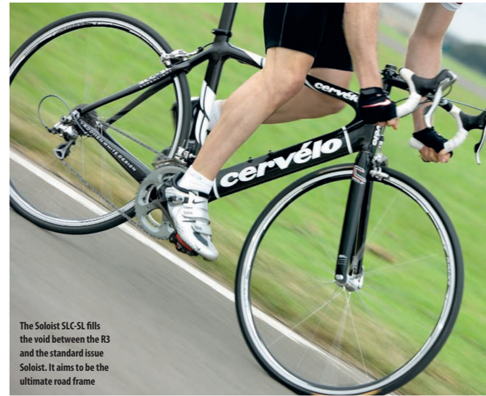
The Cervélo's thin wall tubing has a profile similar to an aeroplane wing
